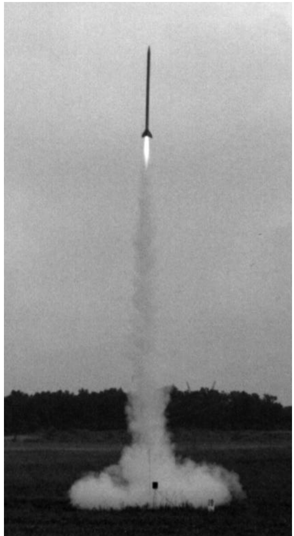
The Sandhawk takes to the skies using an Aerotech Turbo White Lightning hybrid motor.
